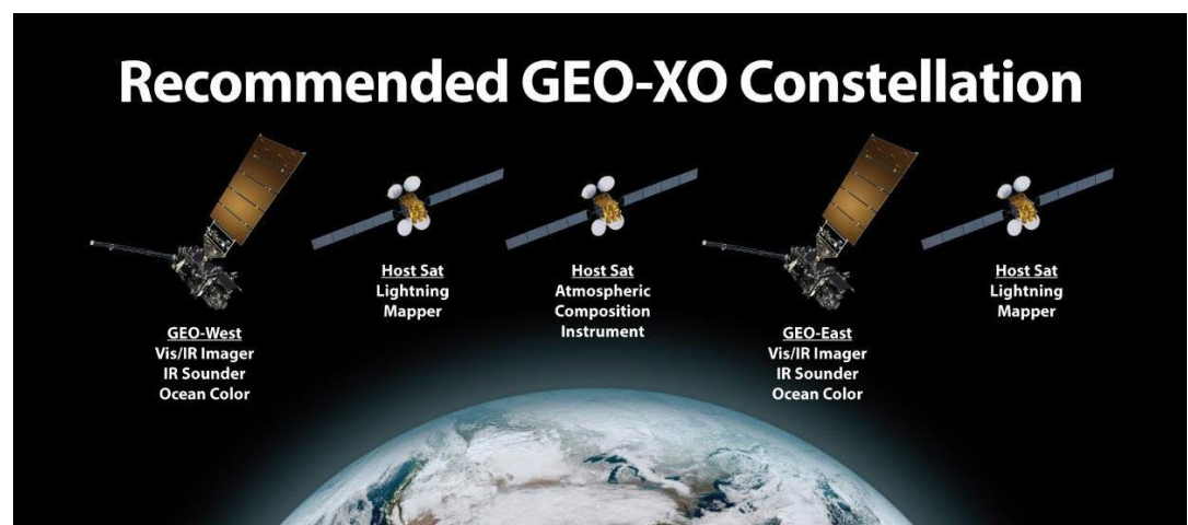
Figure 1: A preliminary proposed GEO-XO constellation concept. (NOAA, 2021)
